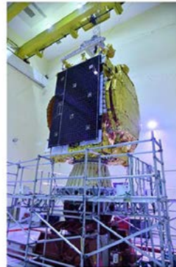
GSAT-N2 undergoing Vibration Test
